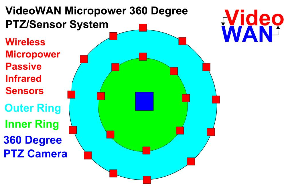
Rings of micropower wireless PIRs trigger the camera's PTZ motors and automatically position the camera for the field of the target and then track it. The motors and analog camera are normally off, using zero battery power. An analog video transmitter is also activated and transmits video to a receiver connected to a network. The system is timed and automatically shuts off. Perpectual operation is possible with solar charging.
